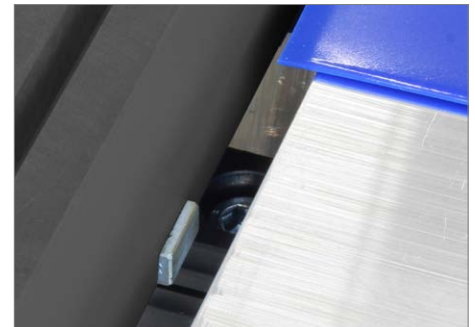
Welding stops for precise repeat welding
