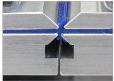
Clamping bars with chamfer for optimum shaping of the welding bead
