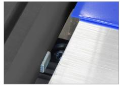
Welding stop for repeatable welds
