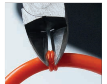
Remove welding bead with side cutter.
