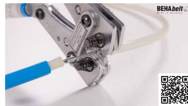
HP01 & CRIMP-Set: For connecting steel-reinforced belt profiles using crimping in the HP01 hot press.
