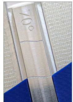
Precise and aligned insertion of the belt ends.
