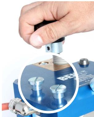
Turn the star handle to the right until the above and lower moulds are touching. Thereafter star handle continue to turn until the screw heads stand 3-4 mm from the upper case plate.
