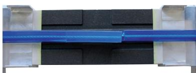
Insert the two ends of the middle and fix it with the clamping screws on the sides. The cutted belt ends lie flush with overlapping.
