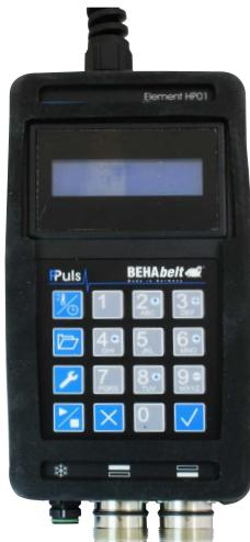
Connect PPuls Controller with the power line and switch on the controller. Selection of welding parameters through direct entry or selection of stored recipes.
