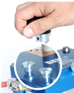
Turn the star handle to the right until the above and lower moulds are touching.
