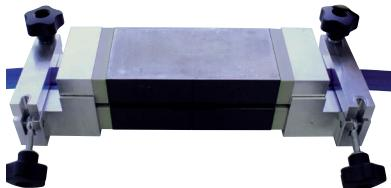
To close the upper part precisely installed on the lower part between the guide webs. During overlap welding the upper part and the lower part initially not touch. The material has yet to be displaced during the welding process or during the holding time.
