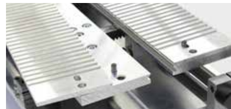
Locking pins ensure that the adapter plates are positioned correctly on the joining table.
