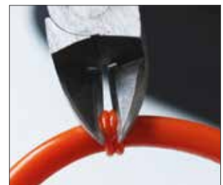
Remove welding bead with side cutter.
