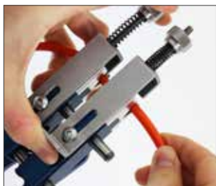
Quick clamp device for inserting the profiles in exchangeable profile jaws.
