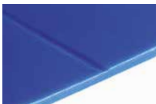
Butt welding with paddle welding tool
