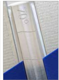
Precise and aligned insertion of the belt ends.
