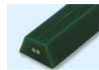
After overlap welding
