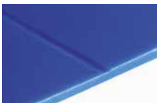
Butt welding with paddle welding tool
