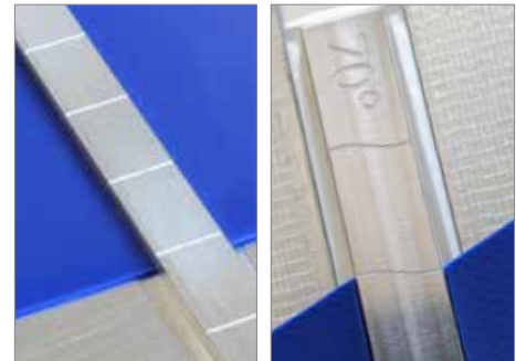
Precise and aligned insertion of the belt ends.
