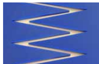
Finger joint with a hot press
