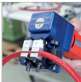
PU and TPE material being processed
