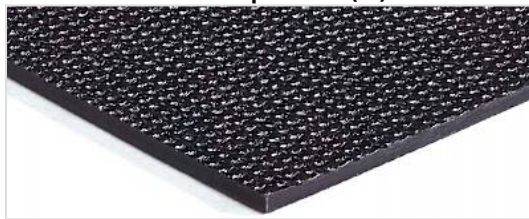
Bottom side: Fabric impression (FI)
