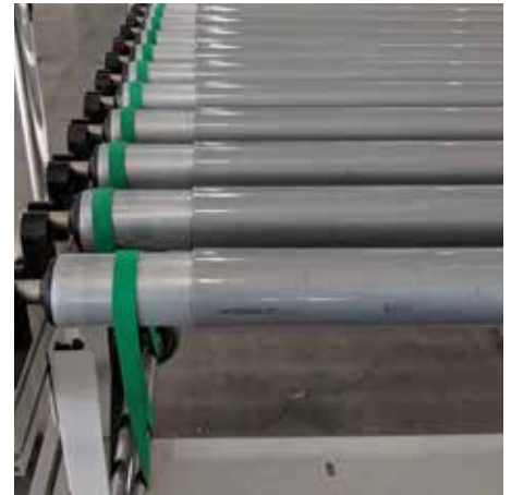
Crossed drive/ Central drive shaft
