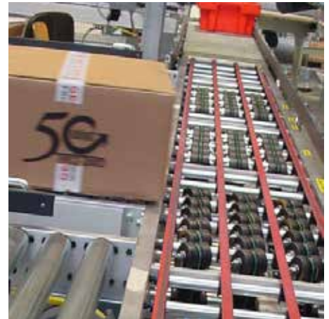
Crossed drive / Central drive shaft
